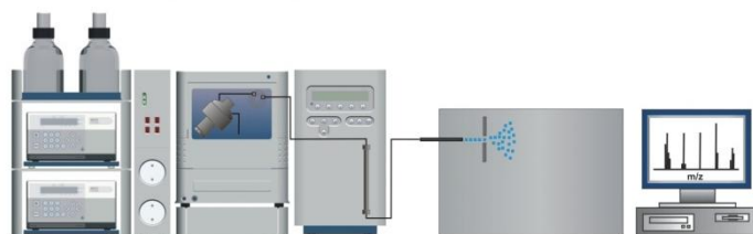
Fig. 1. ROXY™ EC/LC System including ReactorCell™ and AS110 micro autosampler.
