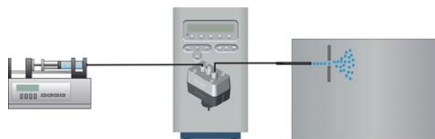
Fig. 3. ROXY™ EC System including ROXY potentiostat, \mu -PrepCell™ and dual syringe pump.
