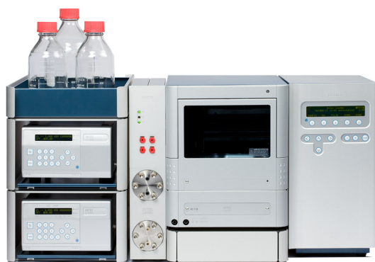
Fig. 1. ALEXYS Aminoglycosides analyzer for Spectinomycin
