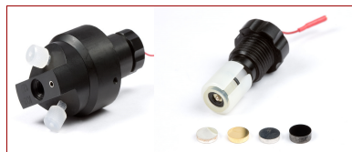
Figure 2: Reactor cell with inlet and outlet (left) and electrode holder with different working electrodes (right).
