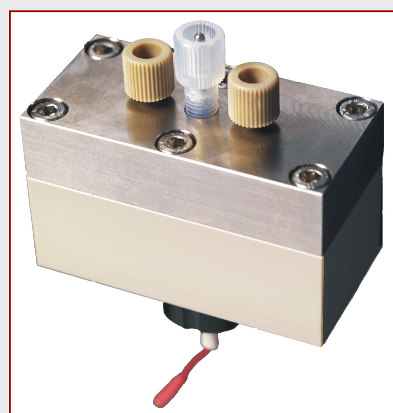
Figure 2: µ-PrepCell ™ with inlet, outlet and reference electrode (top) and working electrode contact (bottom).
