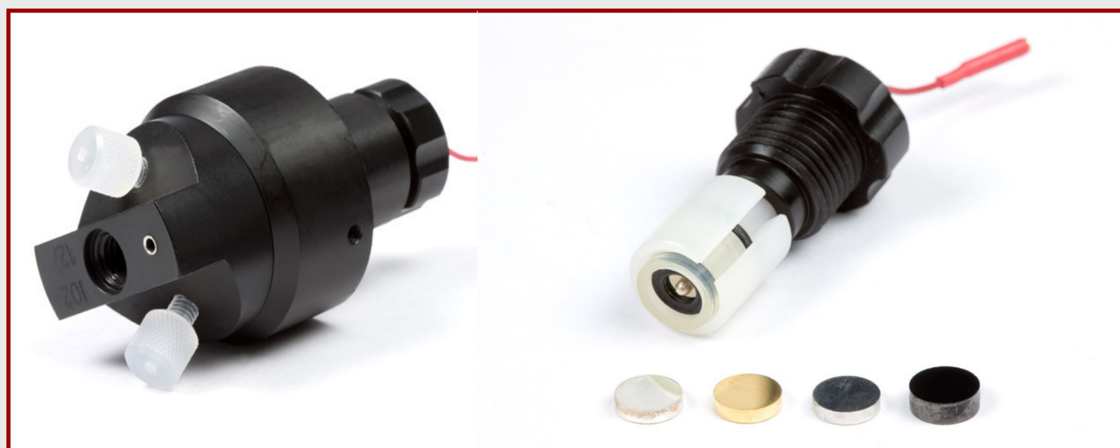
Figure 2: Reactor cell with inlet and outlet (left) and electrode holder with different working electrodes (right).
